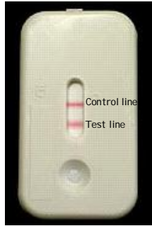
Figure 5: DAS lateral flow test exhibiting a positive result with visualisation of test and control lines
